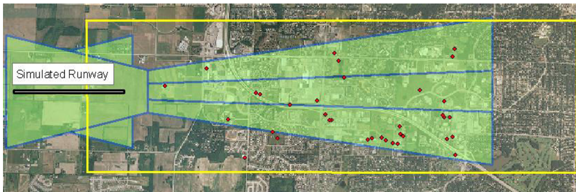
Fig. 7. OIS analysis for simulated runway and ANA LPV approach in southwest Madison project area. The red points indicate locations of field-surveyed reference objects.
