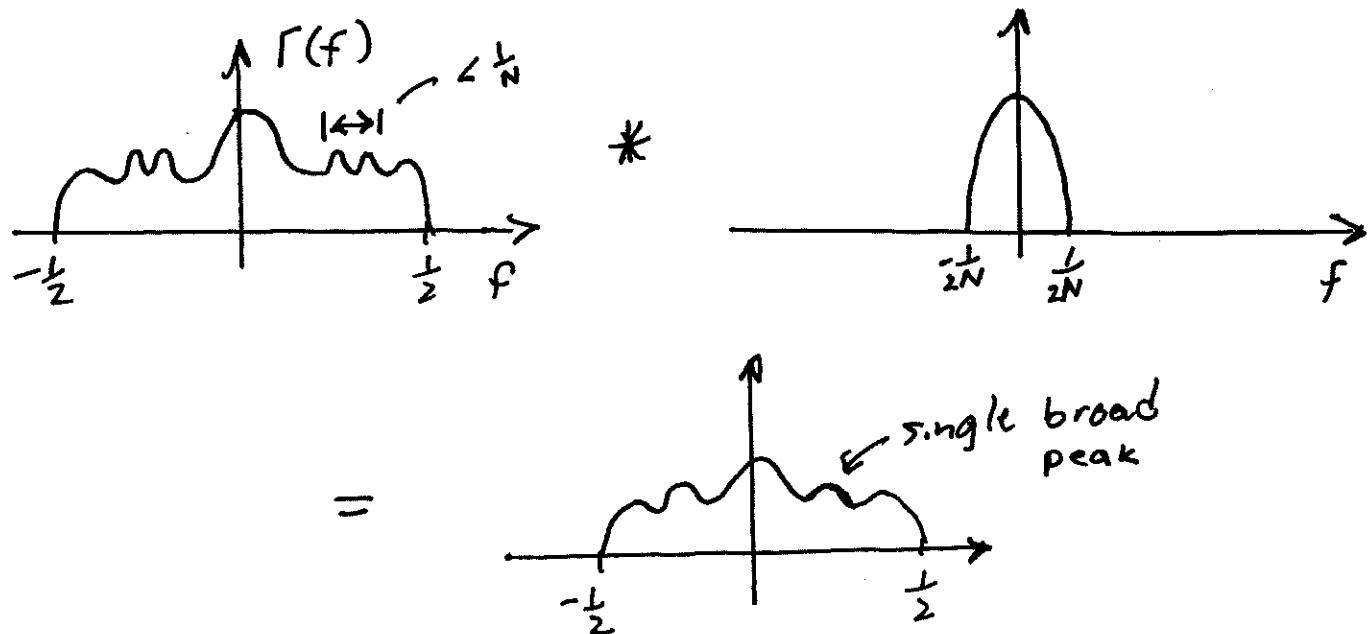
Because of this smearing effect, periodogram estimators cannot resolve details in the spectrum that are separated by less than  $\frac{1}{N}$  Hz. For this reason,  $\frac{1}{N}$  is called the spectral resolution limit of the periodogram.
