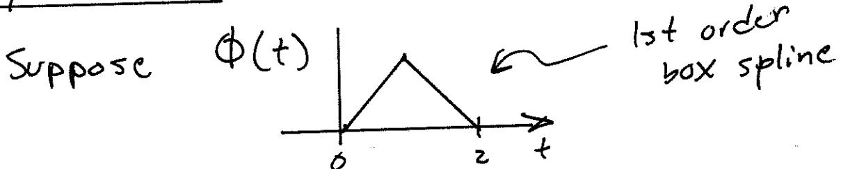
$$\phi(z^j t) = \frac{1}{2} \phi(z^{j+1} t) + \phi(z^{j+1} t - 1) + \frac{1}{2} \phi(z^{j+1} t - 2)$$
