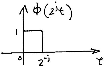
i.e., there exists a func  $\phi(t)$  such that  $\{\phi(z^j t - k)\}$  is a basis for  $V_j$
