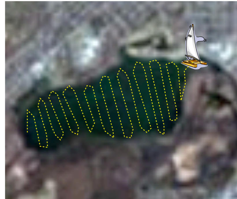
acoustic doppler sensing of water current in Lake Wingra
