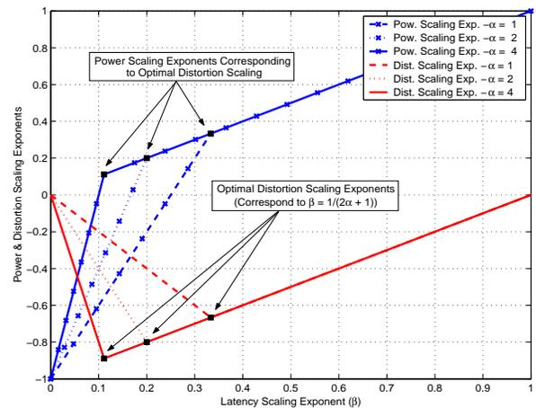
Fig. 3. Power-distortion-latency scaling relationship of compressible signals in the known subspace case. The scaling exponents of  $P_{\text{tot}}$  and  $D$  are plotted against  $\beta \in (0, 1)$  for different values of  $\alpha$ . The filled black square on each curve corresponds to the operating point for optimal distortion scaling ( $\beta = \beta^*$ ), with bias-limited and variance-limited regimes corresponding to the curve on its left and right side, respectively.
