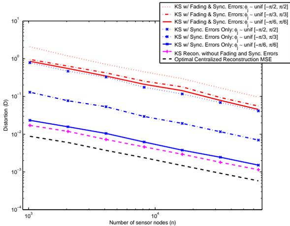
Fig. 9. Distortion scaling of an  $M$ -sparse signal as a function of number of sensor nodes  $n$  under the effects of fading and phase synchronization errors (Known subspace case reconstruction only): number of non-zero coefficients  $M \asymp n^{1/3}$  (in Haar basis); baseline MSE ( $\sigma_w^2$ ) = 1; measurement SNR = 20 dB; received communication SNR per projection = 0 dB; fading envelope: Rayleigh distributed; number of projections  $L = M \asymp n^{1/3}$ .
