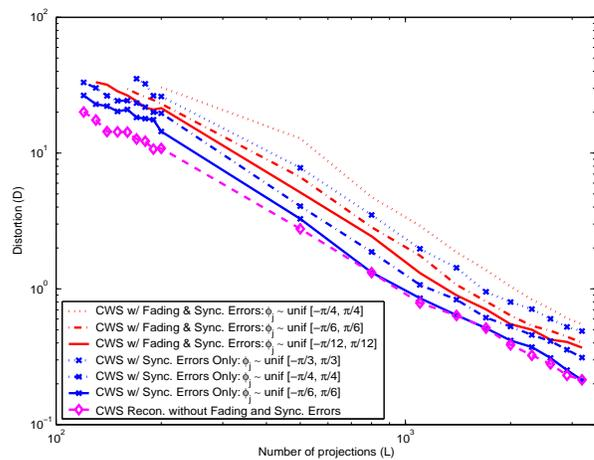
Fig. 10. Distortion scaling of a fixed length  $\alpha$ -compressible signal as a function of number of projections  $L$  under the effects of fading and phase synchronization errors (CWS reconstruction only): number of sensor nodes  $n = 8192$ ,  $\alpha = 1$  (in Haar basis), baseline MSE ( $\sigma_w^2$ ) = 1, measurement SNR = 20 dB, received communication SNR per projection = 0 dB; fading envelope: Rician distributed ( $K$ -factor of 7.5).
