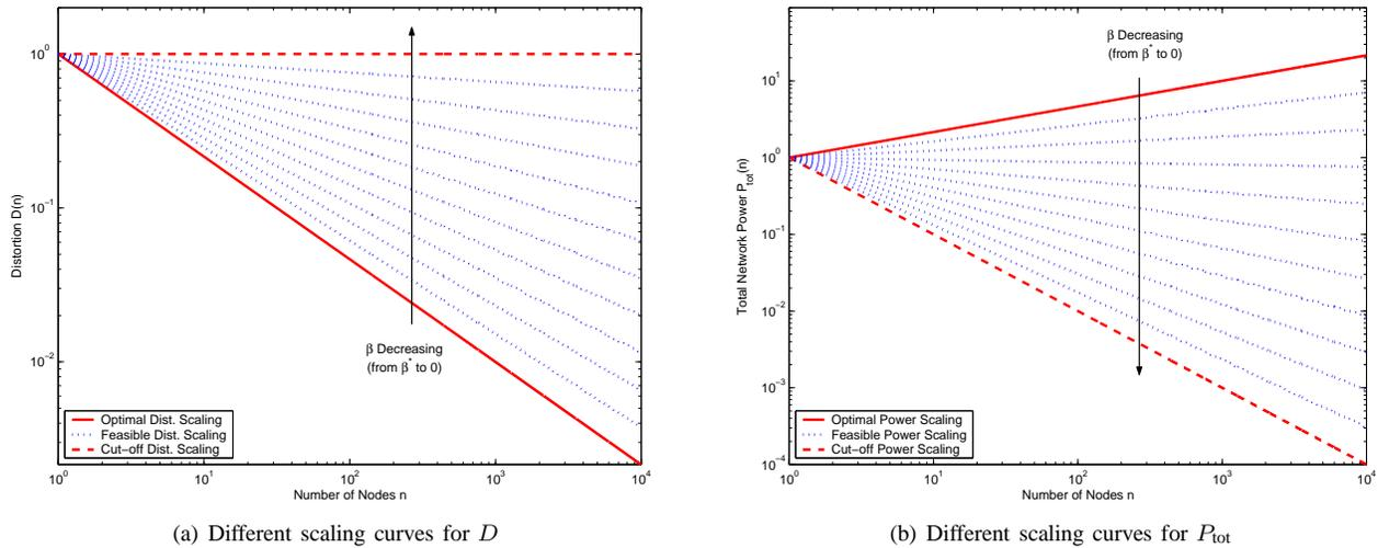
Fig. 4. Power-Density trade-off for compressible signals in the known subspace case. Various power and distortion scaling curves, each one corresponding to a different value of  $\beta$ , are plotted on a log-log scale against the number of nodes for  $\alpha = 1$ . The dashed curves are the cut-off scalings for consistent signal estimation (corresponding to  $\beta \searrow 0$ ).
