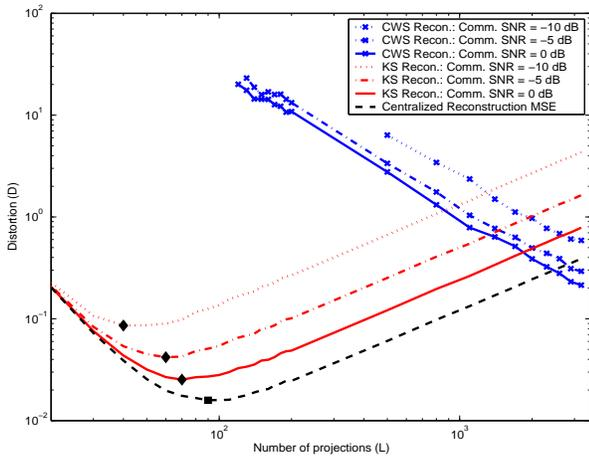
Fig. 7. Distortion scaling of a fixed length  $\alpha$ -compressible signal as a function of number of projections  $L$  for various values of received communication SNR per projection under both known and unknown subspace assumptions (log-log scale): number of sensor nodes  $n = 8192$ ;  $\alpha = 1$  (in Haar basis); baseline MSE ( $\sigma_w^2$ ) = 1; measurement SNR = 20 dB.
