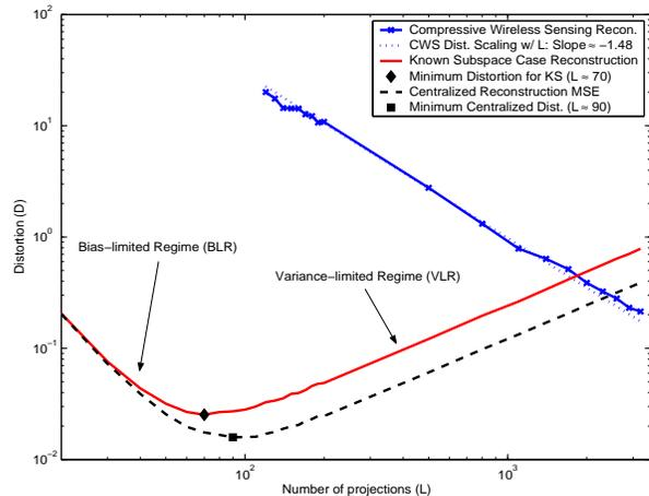
Fig. 6. Distortion scaling of a fixed length  $\alpha$ -compressible signal as a function of number of projections  $L$  under both known and unknown subspace assumptions (log-log scale): number of sensor nodes  $n = 8192$ ;  $\alpha = 1$  (in Haar basis); baseline MSE ( $\sigma_w^2$ ) = 1; measurement SNR = 20 dB; received communication SNR per projection = 0 dB.
